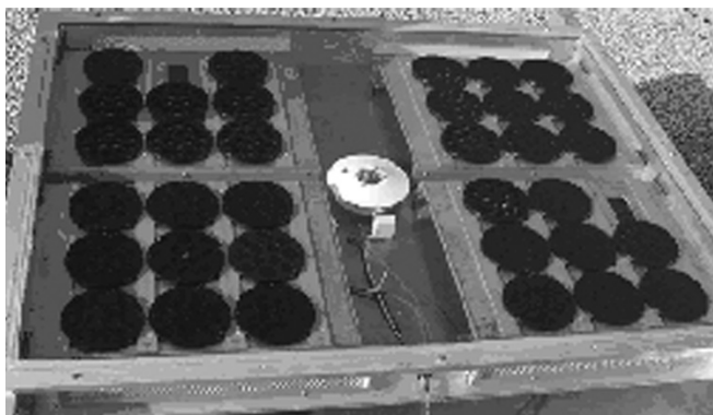
Figure 1—The chamber used for outdoor exposure, showing the exposure cells, the radiometer, and the wires connecting to the temperature and relative humidity sensors.
