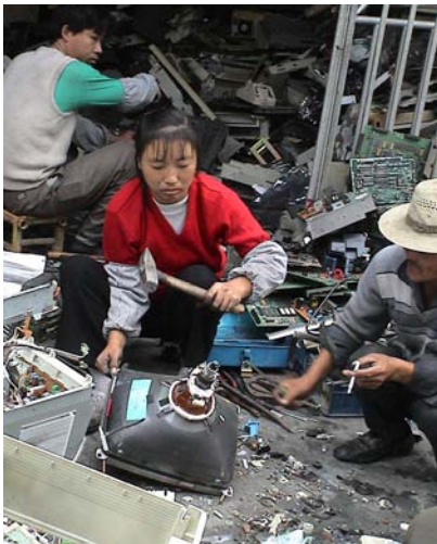
Figure A. Woman about to smash a cathode ray tube from a computer monitor in order to remove the copper laden yoke. Guiyu, China. December 2001. Copyright Basel Action Network.
