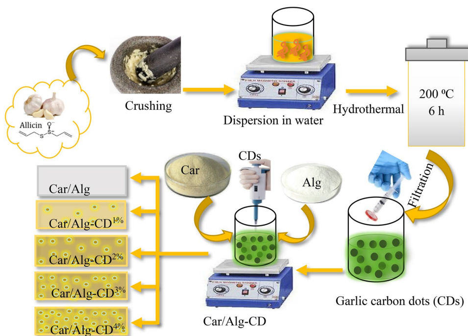
Fig. 1 Schematic illustration of the fabrication of the sodium alginate (Alg), carrageenan (Car), and carbon dots (CD) based Car/Alg, Car/Alg-CD 1% , Car/Alg-CD 2% , Car/Alg-CD 3% , and Car/Alg-CD 4% films
