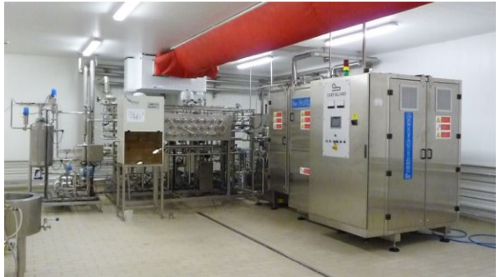
Fig. 1 Tubular heat exchanger (left) and RF equipment (right)
