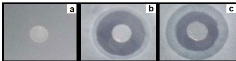
Fig. 5 Diffusion test results of films: with 0.2 g of processed rice bran 100 g -1 slurry (a), with natamycin and nisin (b) and with 0.2 g of processed rice bran, natamycin, and nisin (c), against Saccharomyces cerevisiae and Listeria innocua mixture culture
