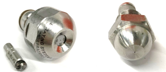
Fig. 2 Pressure swirl nozzles used in this study. Left: SKHN-MFP SprayDry® from Spraying Systems Co.® with outlet orifice diameter of 0.34 mm and corresponding slotted core (No. 16). Right: Schlick 121V from Schlick®, with orifice diameter of 0.3 mm. This nozzle is equipped with a filter to avoid blockage of the nozzle orifice. Preliminary studies showed no influence of the filter on the oil droplet size distribution of the feed emulsion
