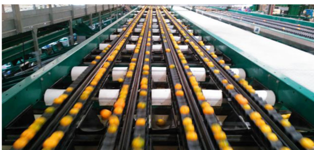
Fig. 5 Commercial electronic sorter for citrus fruits working in a packinghouse
