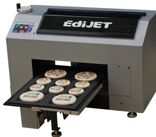
Fig. 1 EdiJET represents an example of an inkjet food printer able to print on several surfaces. Available at http://www.uglyduckclothing.co.uk
