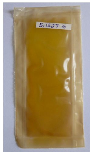
Fig. 1 Sachet for olive oil packaging, produced from emulsified films made of SPI, glycerol, ethanol, SL, and VCO
