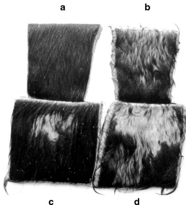
Fig. 4 Dehairing activity of keratinase kr6 on bovine pelts. a Control with heat-denatured keratinase, b keratinase treatment, c and d keratinase treatment followed by gently scrape
