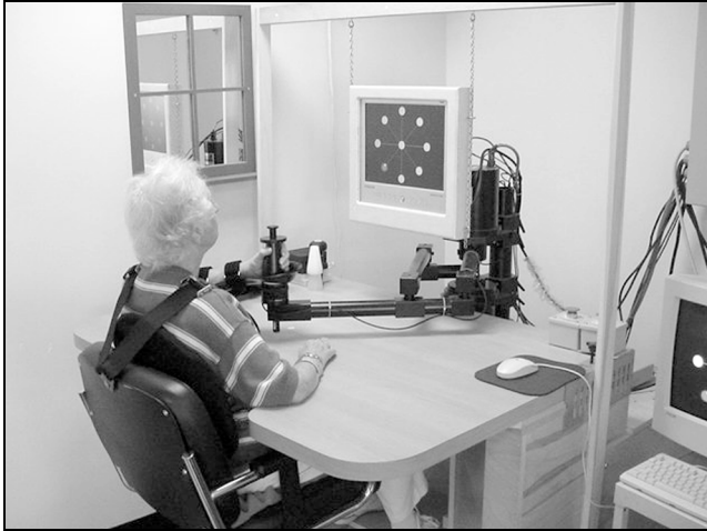
Figure 1. Patient seated in front of the MIT-Manus with her shoulders strapped to the chair and moving the manipulandum. The patient's hand is strapped to a wrist carrier attached to the manipulandum. The video screen is above the training table.
