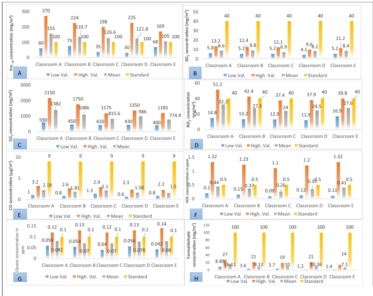
Fig. 4 Concentration of different types of A–H indoor air pollutant in different educational occupancy
