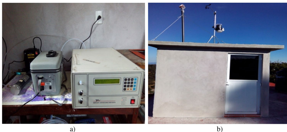
Fig. 3 a Tekran® model 2537A automatic mercury vapor analyzer and b measurement station
