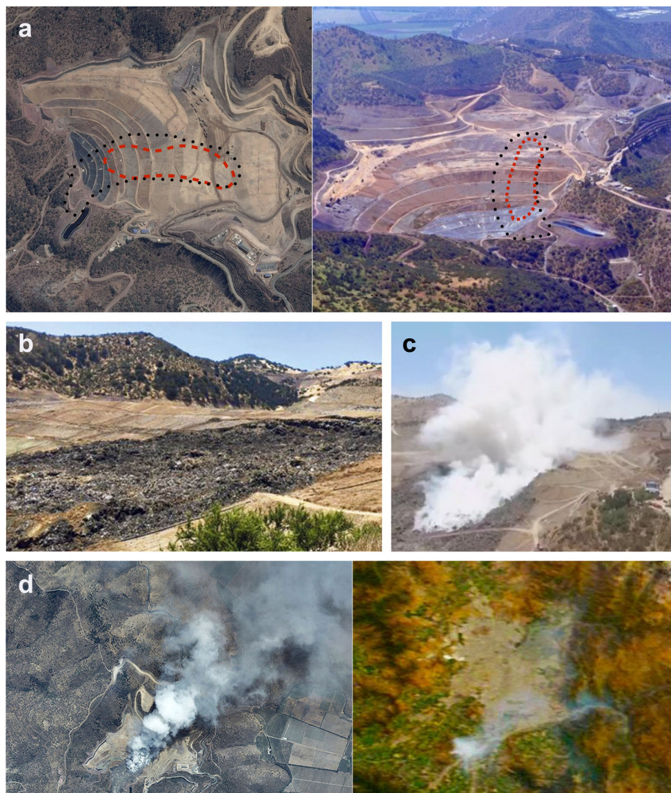
Fig. 3 a Aerial view of Santa Marta landfill. The black line delimits the area of the collapse. The red line delimits the fire zone (source right: google earth v7.1.5.1557, 2016-03-02, Digital Globe 2016. http://www.earth.google.com , accessed 2017-03-10; left: photography Consortium Santa Marta, https://goo.gl/IFxA8m , accessed 2017-03-10). b Side view of the collapsed area of the landfill (source La Tercera Newspaper, https://goo.gl/9vVSeD , accessed 2017-03-10). c Image showing the first moments of the landfill fire (source C13 Broadcast, https://goo.gl/xSJvLi , accessed 2017-10-14). d Aerial and satellite view of the fire smoke plume (NASA, Worldview, 2016-01-19 10:30 AM local time, source: https://worldview.earthdata.nasa.gov , accessed 2017-03-10)
