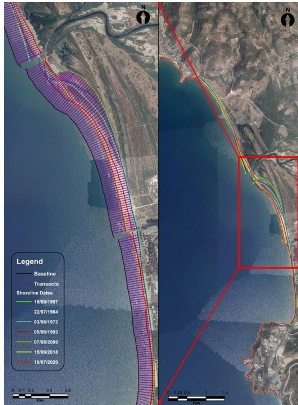
Fig. 3 Multiyear of shorelines, baseline and transect lines on the Küçük Menderes Delta coast
