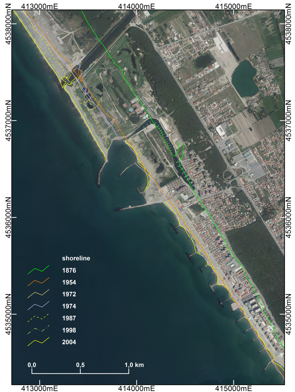
Fig. 12 Shoreline evolution breakwater and downdrift the Pinetamare marina. It is noteworthy the shoreline accretion to north and the beach reduction to south, nowadays stabilized with a dozen of groins
