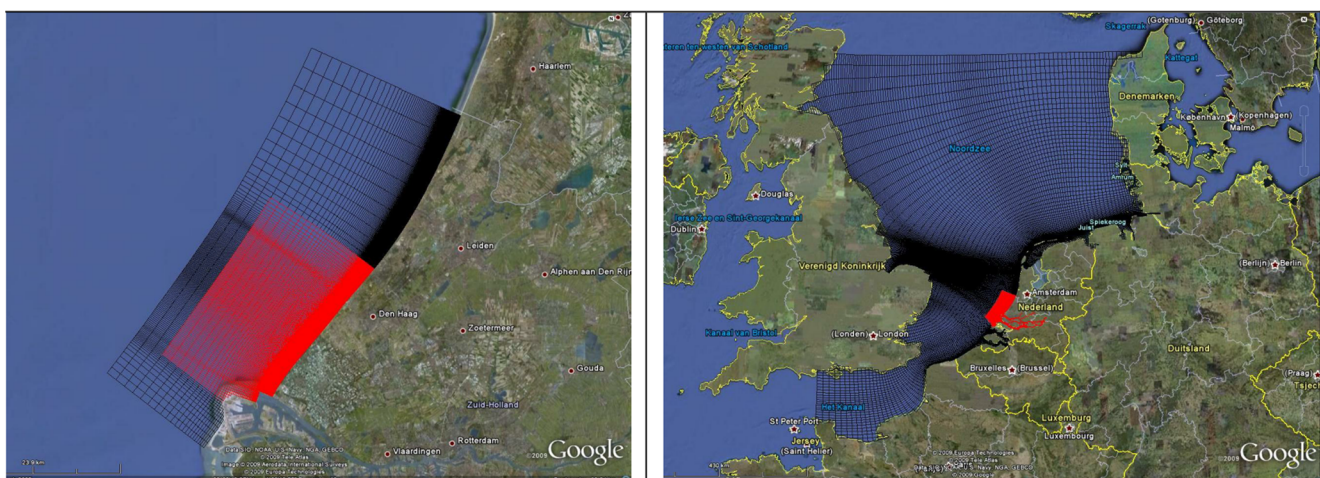
Fig. 6 Left: model domains for flow (red) and wave model (black). Right: ZUNO-FIJN domain (black) and ZEEDELTA v8 domain (red). (From Mulder and Tonnon 2010)
