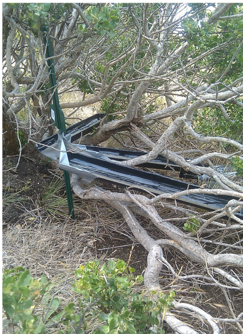
Fig. 4 Fog drip collection troughs placed under shrub cover at the Brazil Ranch study area
