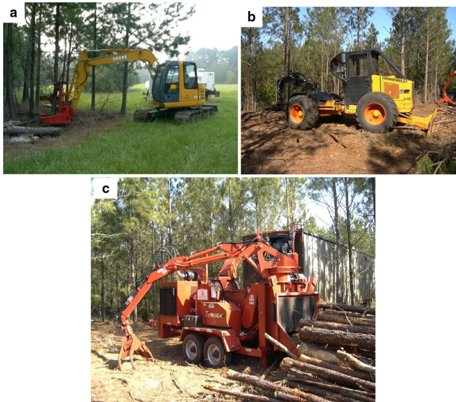
Fig. 1 John Deere 75C with a Fecon shear head (a), Turbo Forest skidder with a grapple attachment (b), Morbark Typhoon chipper with a loader attachment (c)
