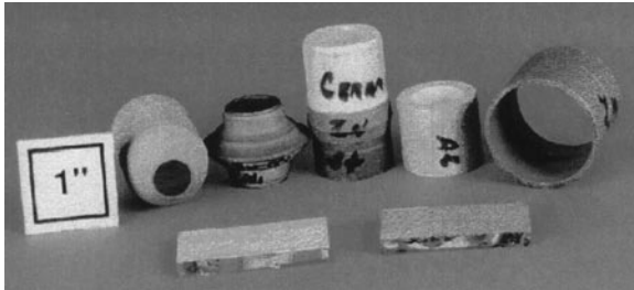
Figure 2. The cold-gas spray method can be used to (a) coat and/or create titanium billets as well as (b) coat alternate materials in a wide variety of shapes and sizes.
