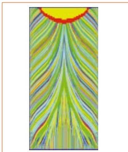
Figure 4. A comparison of calculated and experimental ESR ingot grain structures ( D = 432 mm, 272 kg/h, H = 2.1 m, 16 million microvolume elements, CPU time = 10 hours). (a) The experimental initial transient state, (b) the calculated initial transient state, (c) the experimental steady state, (d) the calculated steady state, (e) the experiment final transient state, and (f) the calculated final transient state. The macroetches of the ESR ingot were scanned from Reference 25.
