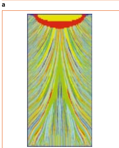
Figure 5. The grain structure formation of VAR alloy 718 ingots ( 172 kg/h, D = 508 mm) (a) without fluid flow and (b) with fluid flow.
