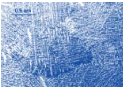
Figure 7. A micrograph of an alloy 625 freckle within an ingot-equiaxed solidification zone.
