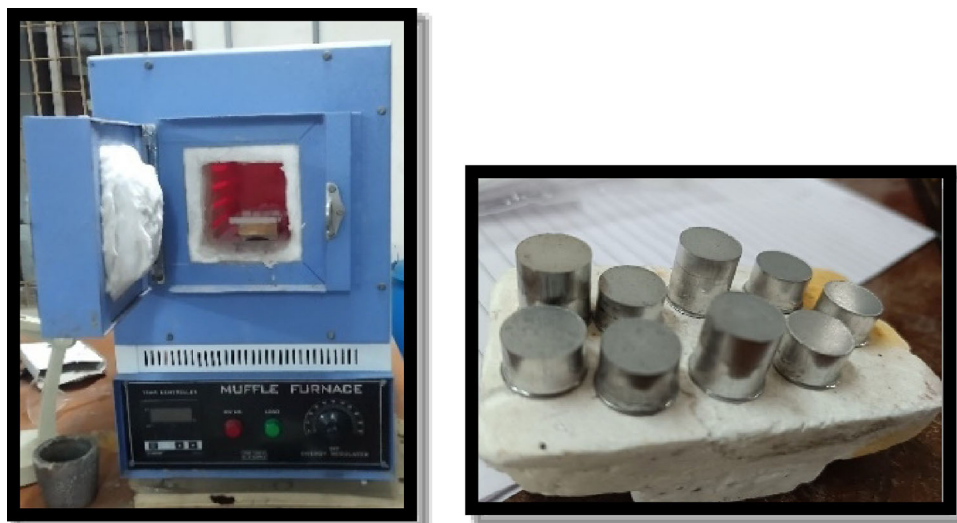
Fig. 3. (a) Muffle furnace; (b) composite samples.
