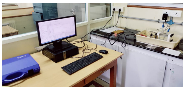
Fig. 4. Apparatus for polarization test.
