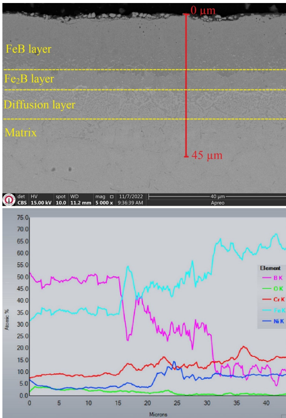
Fig. 2. Section analysis of the boride layer obtained on the surface of AISI 316 steel because of boriding at 900°C for 2 h: SEM view and EDS line analysis.
