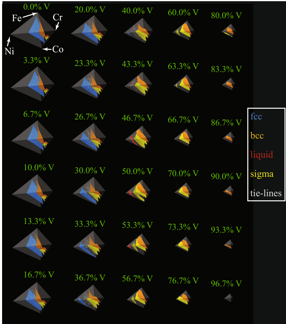
Fig. 5. Example of interactive exploration of the Co-Cr-Fe-Ni-V phase diagram (1500 K isothermal section). Surfaces indicate phase boundaries, color coded by phase, while tie-lines are shown in white. The image sequence starts at the top left with the Gibbs tetrahedron associated with the Co-Cr-Fe-Ni system and the remaining image sequence shows (from top to bottom and then left to right) cross-sections of constant V concentration with V content gradually going from 0 to 100 at% in successive images.
