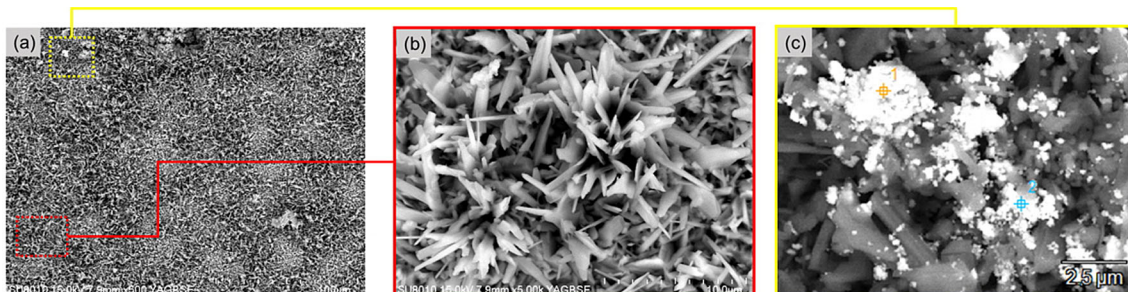
Fig. 6. Top-view images of the PC800_5h_O specimen, which was pack-cemented at 800°C for 5 h and subsequently oxidized at 1000°C for 3 h: (a) overall image of the specimen after oxidation without any sample preparation, (b) magnified image of the Al oxide region with points where the region was analyzed using EDS point analysis, and (c) magnified image of the HEA oxide region with points where the region was analyzed using EDS point analysis.
