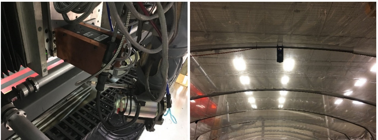
Fig. 2. Example sensing equipment. The left image shows a Keyence laser profilometer, while the right image shows a FLIR thermal camera.
