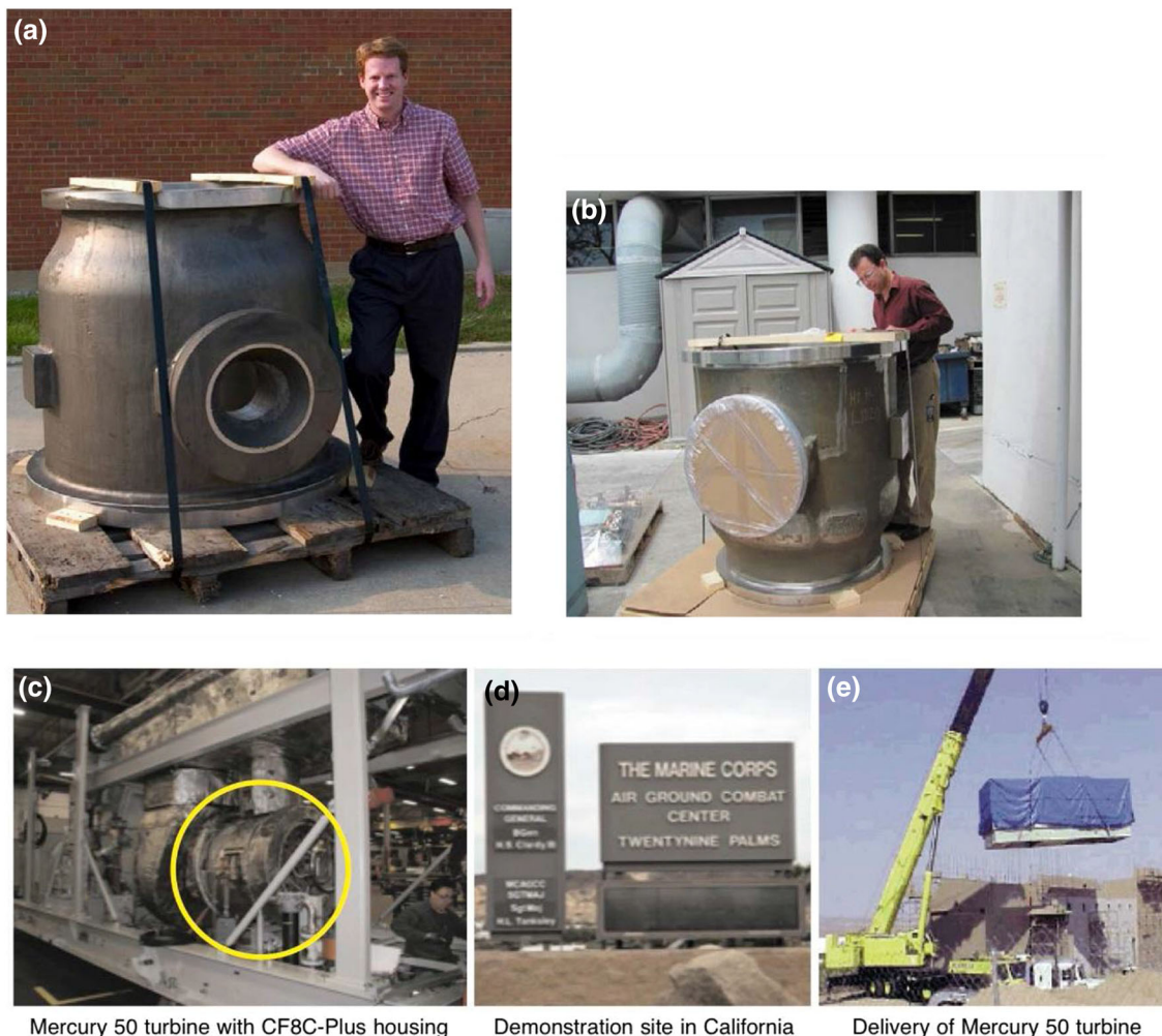
Fig. 9. A Mercury 50 gas turbine engine end cover (6700 lb) cast in 2005 by MetalTek International for Solar Turbines and sent to the Caterpillar Technical Center for destructive analysis and then a second end cover cast for deployment on a Mercury 50 gas turbine in 2011 and installation (29 Palms Marine Base in California) in 2013, which has operated successfully since 2014. 18 (Reprinted from Ref. 18).
