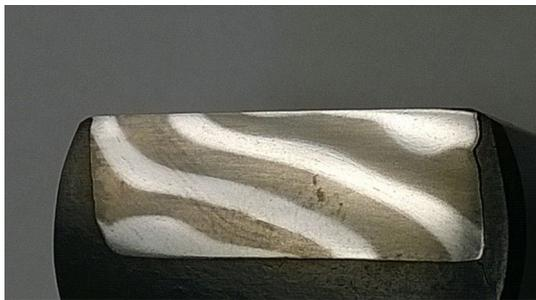
Fig. 7. Macrograph of layered steel.
