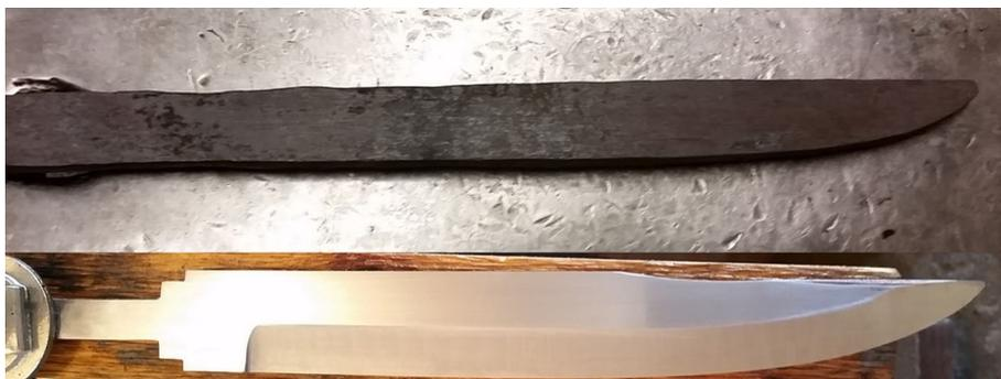
Fig. 4. Top Forged blade, bottom semi-finished blade.
