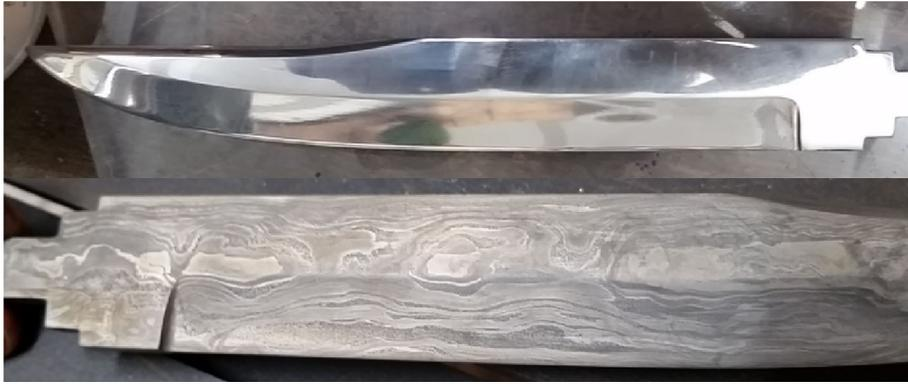
Fig. 6. Top Blade prepped for etching, bottom etched blade revealing pattern.
