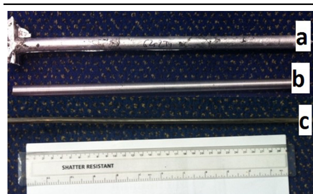
Fig. 1. Cast (a), machined (b) and rolled (c) billets of MA2.
