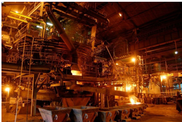
Fig. 1. Photo of the FeMn furnace during tapping.
