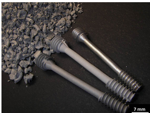
Fig. 2. Bone screw demonstrator made with Mg-0.9Ca feedstock using MIM. Parts (bottom to top) green part after MIM, solvent debond green part and sintered part.
