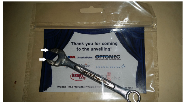
Fig. 6. Stainless steel crescent wrench repaired with the LENS Hybrid CNC Vertical Mill.
