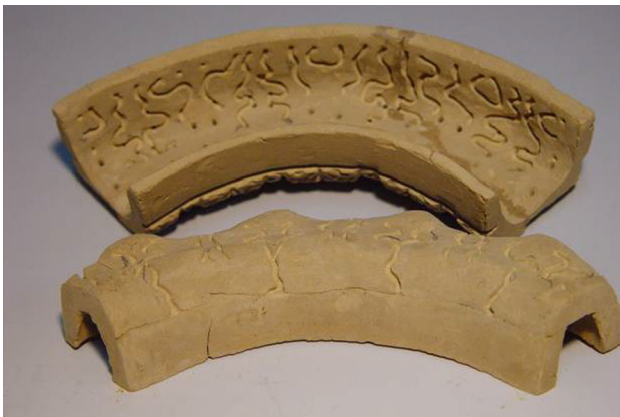
Fig. 7. Second set of pouring channels on the inner core mold for casting the zun.
