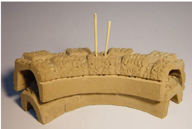
Fig. 6. Pouring cross-channels formed by piercing holes for casting the zun.
