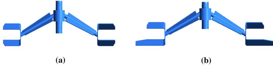
Fig. 2. Geometry of the Intermig impellers: (a) structure of upper impeller and (b) structure of lowest impeller.
