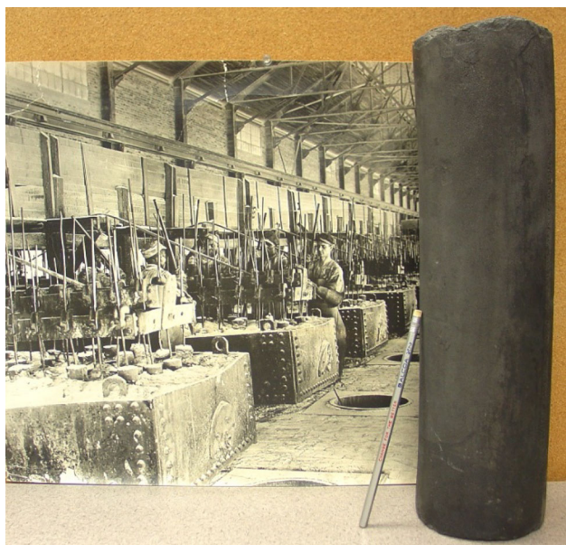
Fig. 1. Early generation Alcoa Tennessee anode (5" diam. × 18" long) in foreground with potroom photo in background (courtesy Steve Lindsay, Alcoa).
