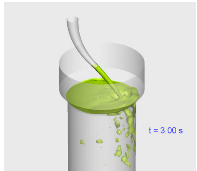
Fig. 2. The top surface fluctuation and gas entrainment in a mold during centrifugal continuous-casting process.
