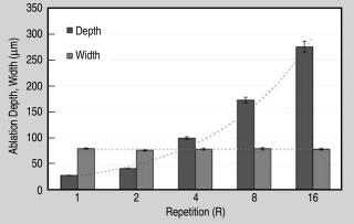
Figure 6. The relationship dimensions of micromachined material (ablation width, ablation depth) and repetition (1x, 2x, 4x, 8x, and 16x)at constant aperture size for ArF laser micromachining of Si (111). Data is expressed as mean  $\pm$  standard deviation (P<0.05).
