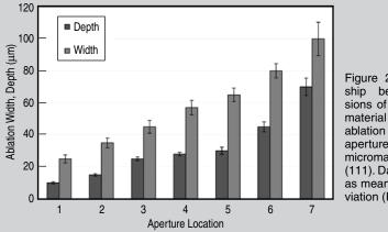
Figure 2. The relationship between dimensions of micromachined material (ablation width, ablation depth) and aperture for ArF laser micromachining of Si (111). Data is expressed as mean  $\pm$  standard deviation (P<0.05).
