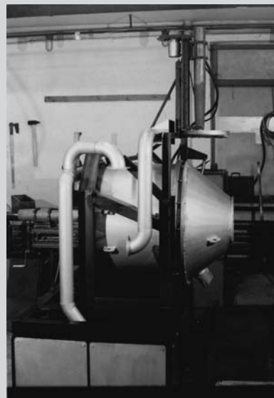
Figure A. A DC electric arc rotary furnace with a displaced 90° electrode.
