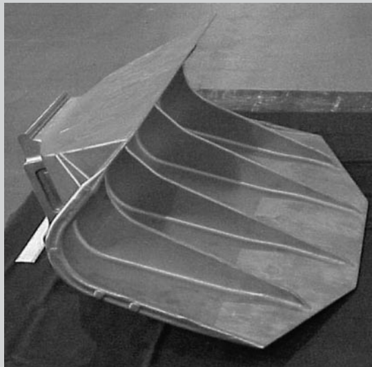
Figure 5. A 33 cm × 86 cm × 127 cm slab cast in the furnace shown in Figure 4. 8
