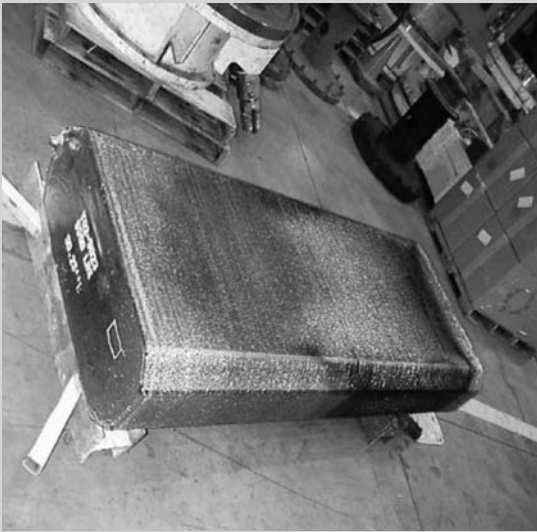
Figure 5. A 33 cm × 86 cm × 127 cm slab cast in the furnace shown in Figure 4. 8
