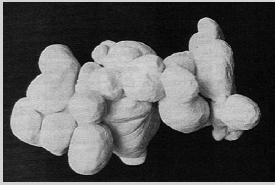
Figure 5. A 3-D reconstruction showing the interconnection of single agglomerate. 5
