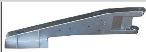
Figure A. An investment cast Ti-6Al-4V stabilizer arm (approximately 39.9 cm wide, 194.6 cm long, and 45 kg).
