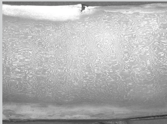
Figure 2. Alwar bar 3 after forging to 5 mm thickness, width = 42 mm.
