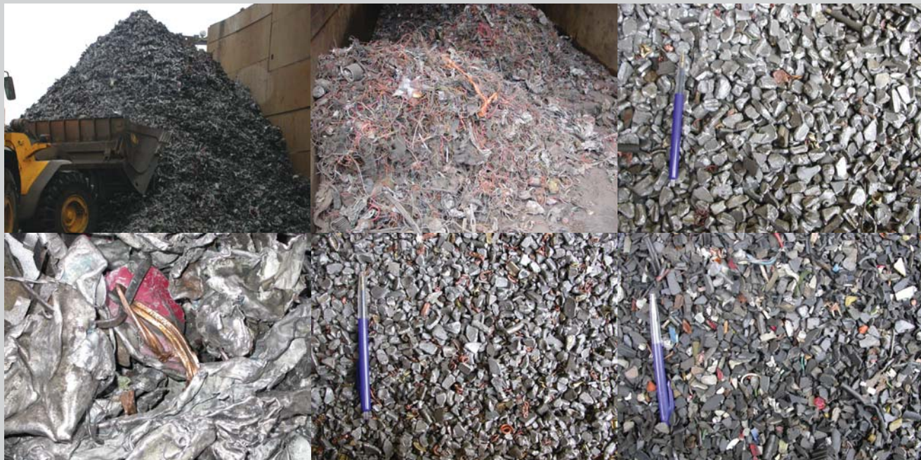
Figure 1. The diverse and distributed properties of recycling materials (clockwise: steel approximately 650 t. from 1,153 ELVs; copper fraction; Al/Mg/Cu/Zn fraction; plastic fraction; Al/Mg/Cu/Zn fraction; steel fraction).
