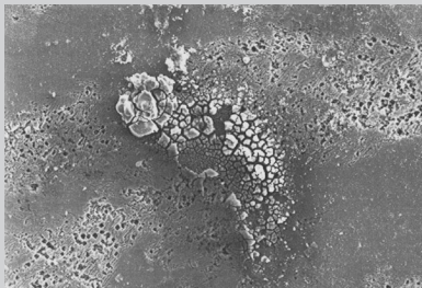
Figure 11. The formation of gelatinous \text{Al}(\text{OH})_3 in the form of mothballs and its cracking.
