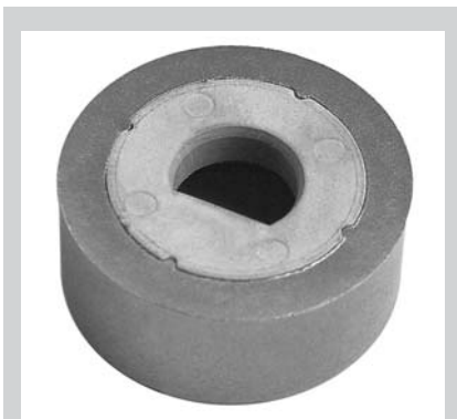
Figure 4. Despite the lack of a gap between the alumina and austenitic stainless-steel regions of this component, which was two-color injection molded, debound, and vacuum sintered, bonding between the two regions was poor.
