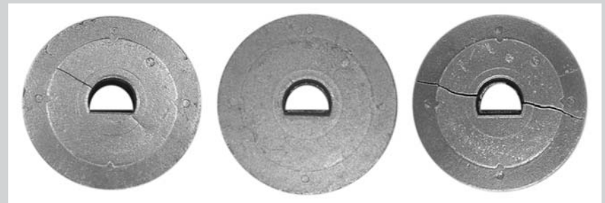
Figure 8. The radial cracking of stainless-steel components consisting of ring materials with different relative shrinkages. The shrinkage of the outer ring of the left component was too low, while the shrinkage of the outer ring of the right component was too high.
