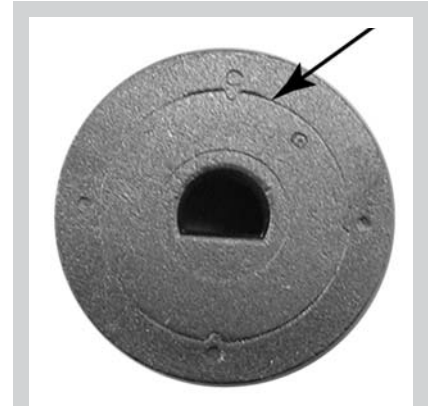
Figure 3. The interfacial separation (indicated by arrow) between an outer austenitic stainless steel ring and an inner ferritic stainless steel ring, which were two-color injection molded, debound, and vacuum sintered.
