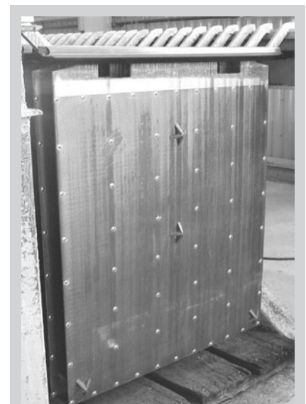
Figure 1. A photograph of a Mesh-on-Lead anode prior to testing.
