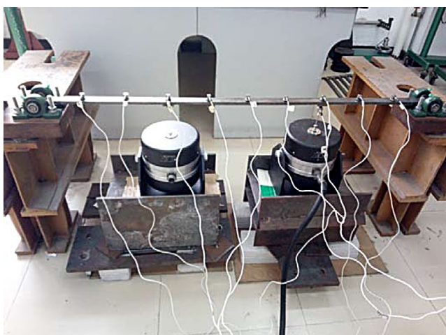
Fig. 14 Experimental model of a laboratory-scaled steel beam [127]
