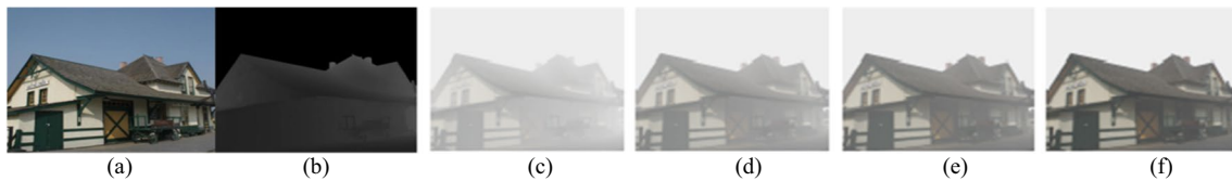
Fig. 24 HazeRD samples from left to right, a Haze-free image, b depth map, simulated hazy images with the visual range of c 50 m, d 100 m, e 200 m, and f 500 m, respectively
