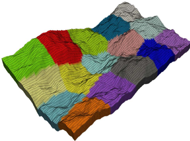
Fig. 8 Partition of a reservoir model into subdomains
